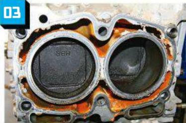
the photo. Glopping usually occurs when air is in the coolant system and corrosion occurs on the aluminum parts in the engine. Coolant then washes over the corrosion, causing a glopping effect to occur. Using a phosphate and silicate-free coolant is the best solution for most aluminum engines.
