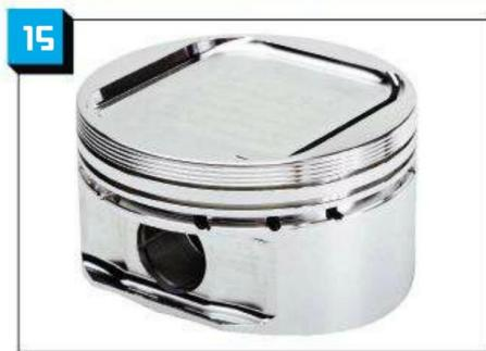
**16** Similar to our connecting rod, each JE piston was carefully weighed and machined to perfectly match weight for all four.
