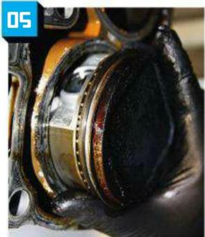
walls while a more severe case of scoring can be caused from heat seizing. The case of peppered markings or indentations across the tops of the pistons indicates detonation/pinging, while a melted piston is caused from an excessively lean air/fuel ratio.
